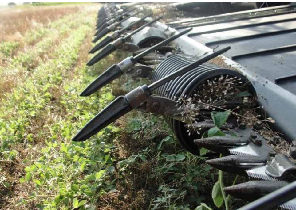
A low-cost solution for relay-cropping. Covering cutter bar with tile pipe; Rutland, ND.
